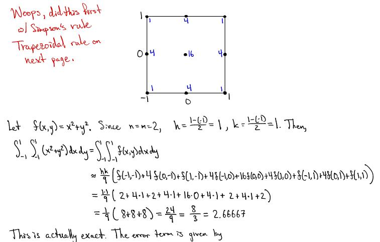
$$E = -\frac{(d-c)(b-a)}{180} \left[ h^4 \frac{\partial^4 f}{\partial x^4}(\eta, \mu) + k^4 \frac{\partial^4 f}{\partial y^4}(\eta' \mu') \right]$$
